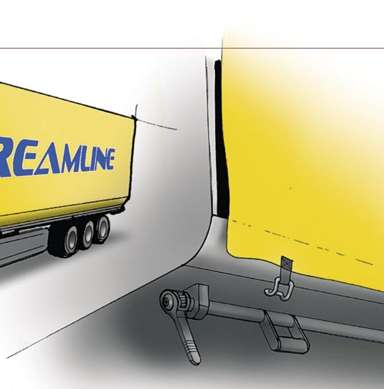
In stead of copying the present tapes of 50 millimeters width, the strengthening yarns can be laid over a larger area. At the thinner sections of the tarpaulin, the material will bend more easily. Thus generating a regular folding pattern for the side curtain. The rollers for the top rail system can be mounted in these reinforced sections.
